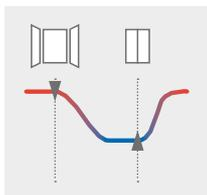
Open window detection: radiator automatically switches off if a window is open for an extended period.
